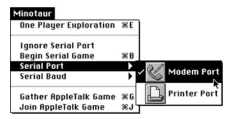
A serial port's baud rate is proportional to the speed at which information is transmitted. Minotaur sends very little information through the serial port and will run at nearly the same speed at all baud rates. In general, however, it's a good idea to play at the highest baud rate possible.
